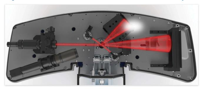
Patented tri-laser design utilizing all red lasers, all blue lasers or a combination. These different configurations give better accuracy depending on the size of your particles.
